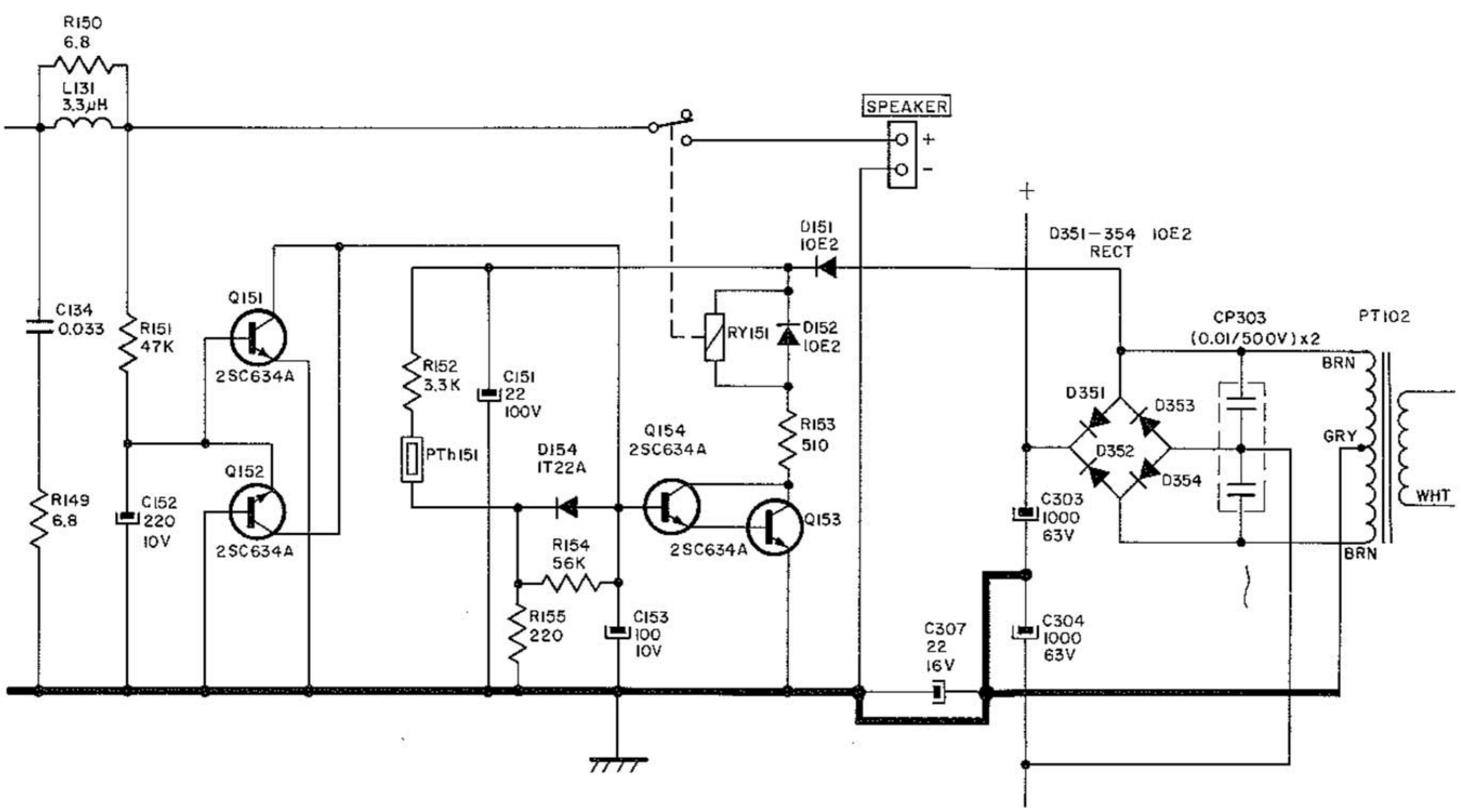
Fig. 6. TA-N7B Speaker Protection Circuit
