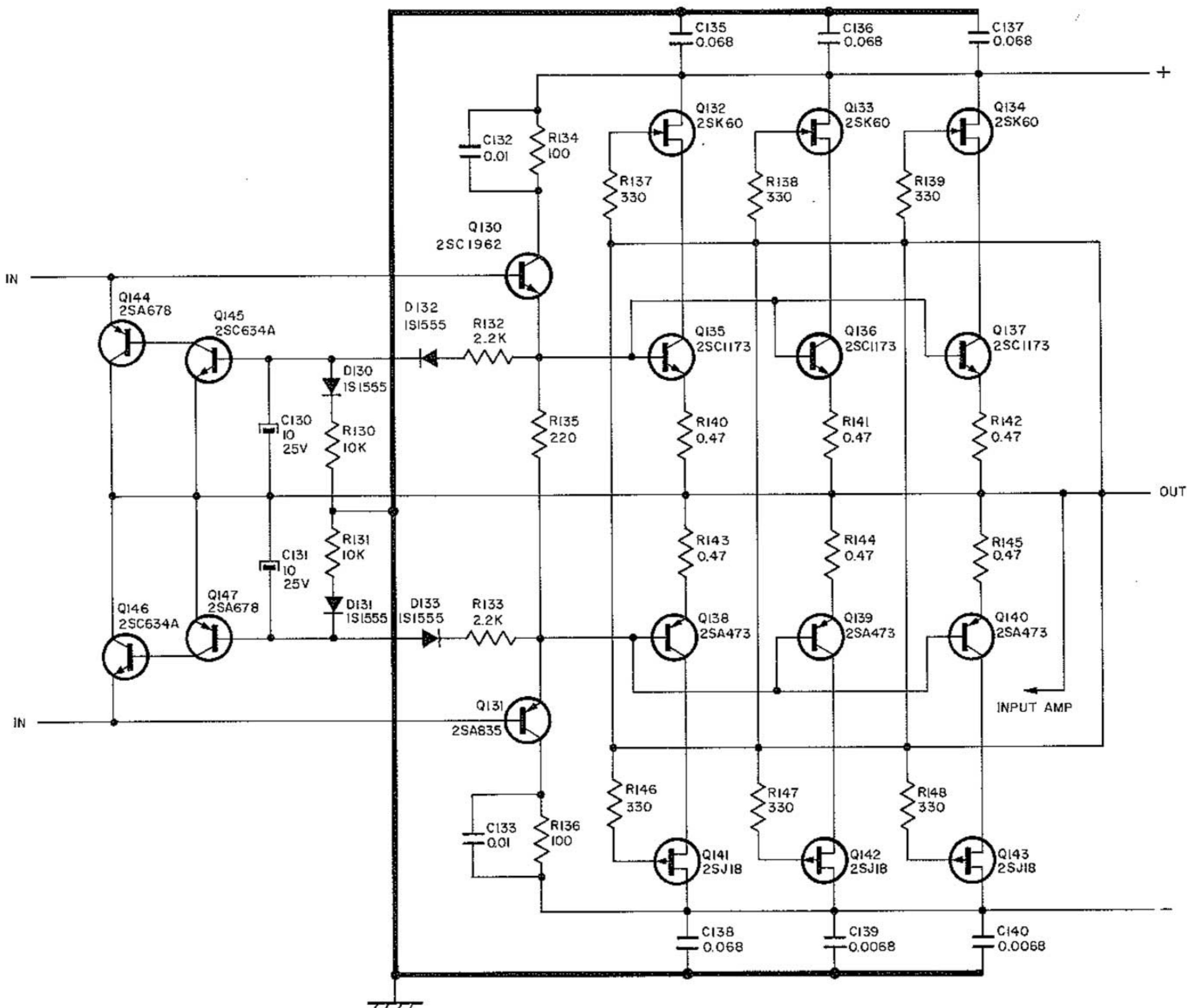
Fig. 3. TA-N7B Power Output Stage
