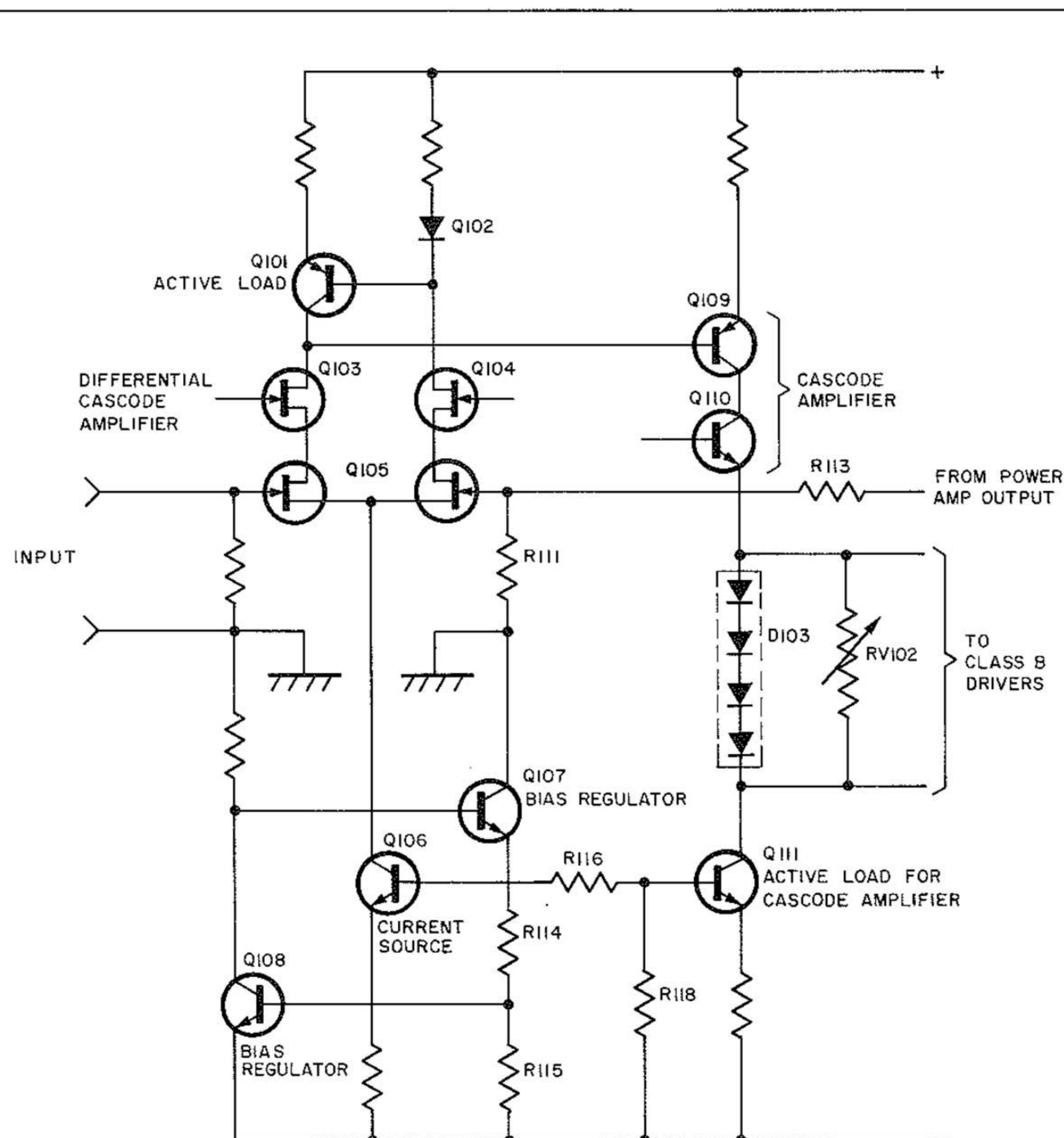
Fig. 2. TA-N7B Simplified Schematic of Input Amplifier
