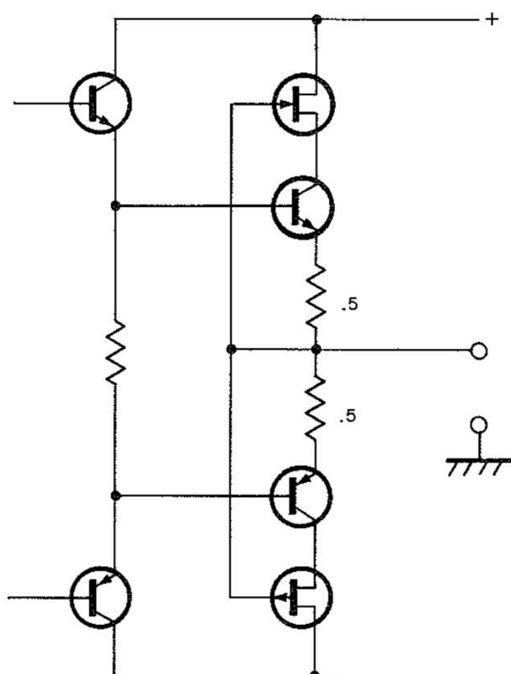
Fig. 4. TA-N7B Simplified Schematic of Power-Output Stage
