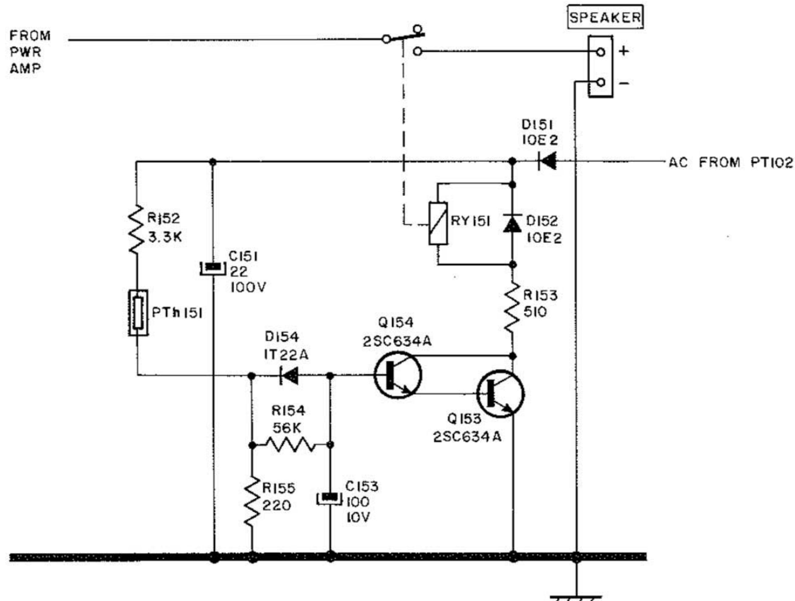
Fig. 5. TA-N7B Thermal Protection Circuit
