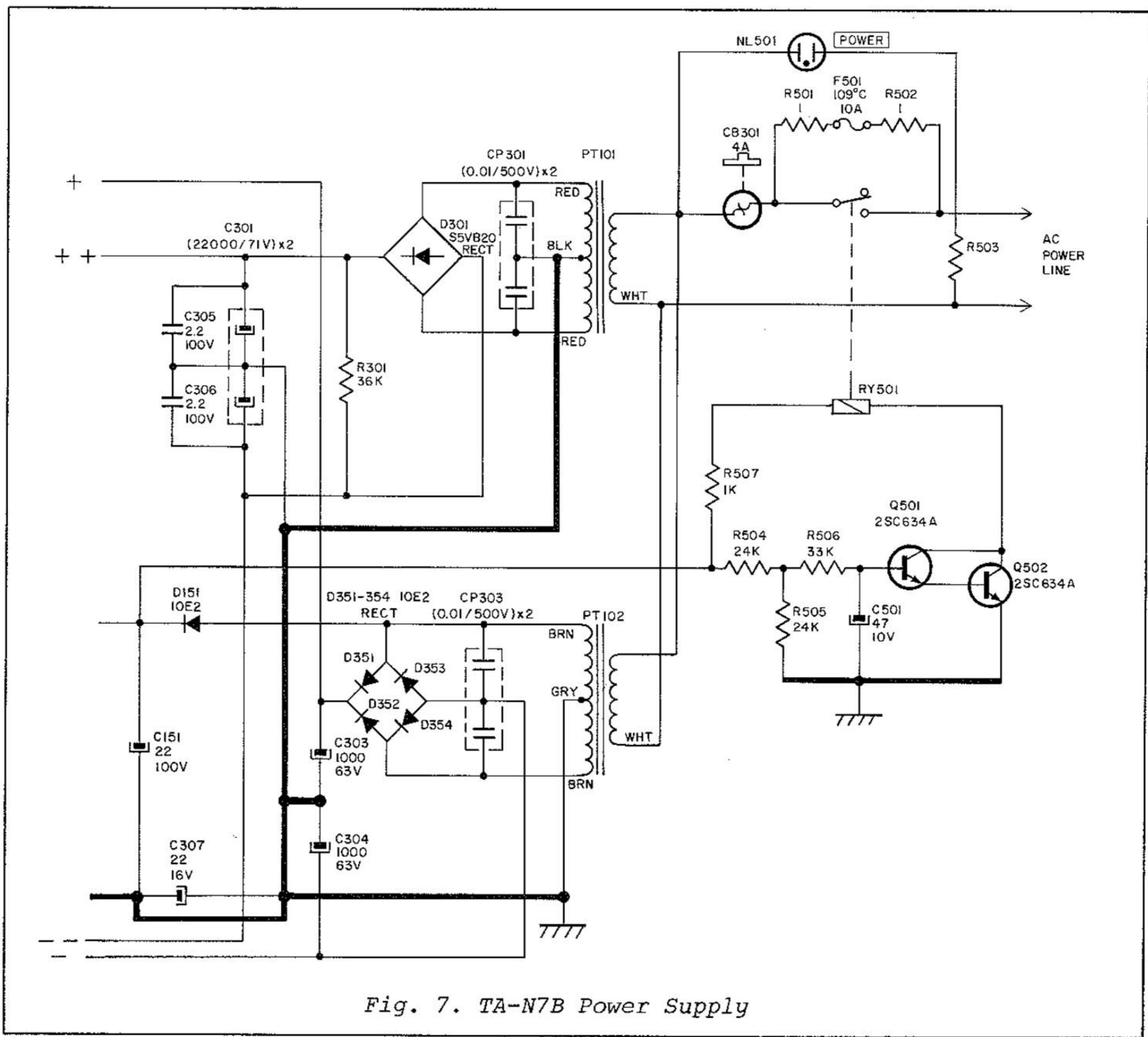
Fig. 7. TA-N7B Power Supply
