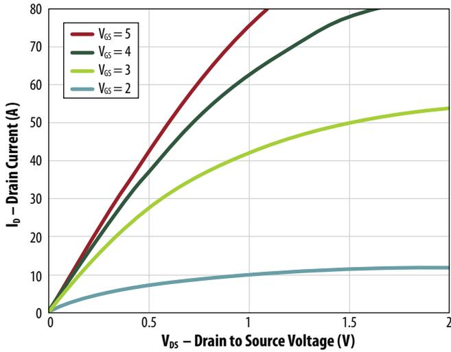
Figure 2: Transfer Characteristics
