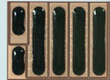
EPC2016 eGaN® FETs are supplied only in passivated die form with solder bars
