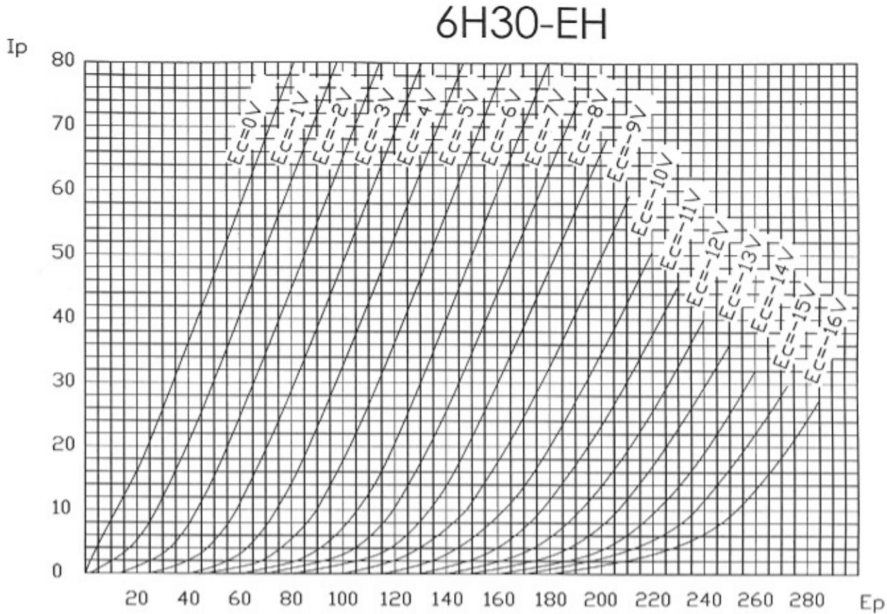
The 6H30 is a medium-mu dual triode with a very high-pervance cathode. The low plate resistance, combined with superior linearity, and a true 4 watt per plate dissipation, make for a high performance voltage amp or driver.
