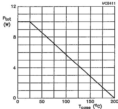
Fig.2 Total power dissipation as a function of case temperature.
