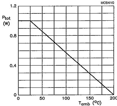
Fig.3 Total power dissipation as a function of ambient temperature.
